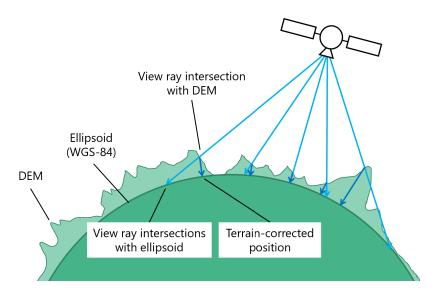
A *rectification* is the transformation of satellite imagery from its original viewing geometry into a target geometry that forms a regular grid in a defined coordinate reference system (CRS) with uniform spatial resolution for each pixel in each dimension. For the Sentinel-3 OLCI Level-1b scene above, the rectified measurement image for the geographic projection (CRS EPSG:4326) is shown here:
