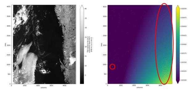
The given coordinates, latitude and longitude, are *terrain corrected* with respect to a digital elevation model (DEM) that approximates the Earth's true fractal surface. Therefore, the gradient vectors are not monotonically varying over the scene, instead they represent the roughness of the DEM. Areas of high surface roughness are indicated by the red circles in the figure above. The figure below should explain the cause of the effect.
