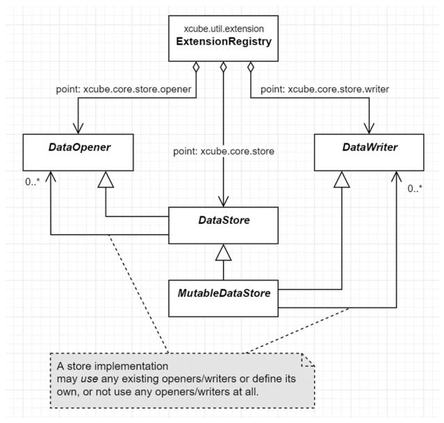
Here, we implement a dedicated DataOpener for a suitable combination of supported Python data types, external storages types, and/or data formats. The DataStore, which implements the DataOpener interface delegates to specialized DataOpener implementations based on the open parameters passed to the open\_data() method. The same holds for the DataWriter implementations for a MutableDataStore.
